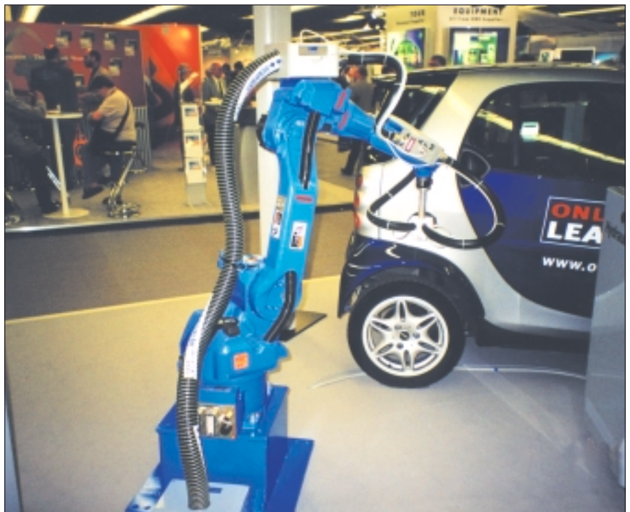
Robotic fueling system developed by JRS GmbH.
